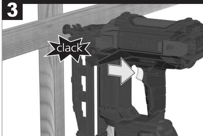
Switch to single sequential actuation
