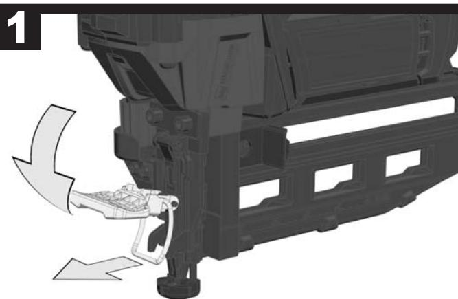
Clearing a Jammed Fastener
